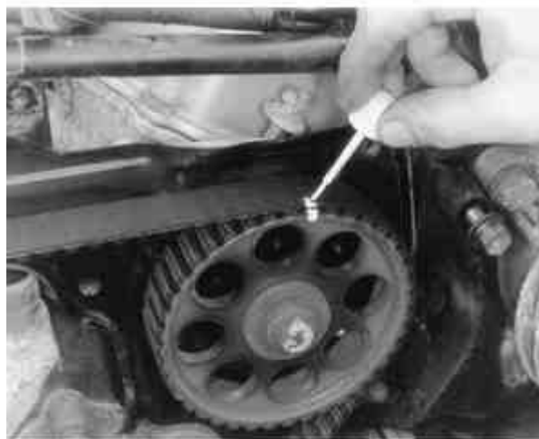
Fig. 15: Release the timing belt tensioner assembly
