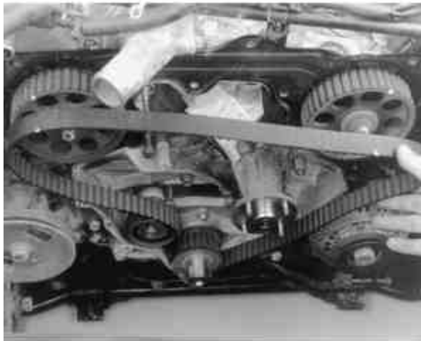
Fig. 17: Removing the water pump mounting bolts
