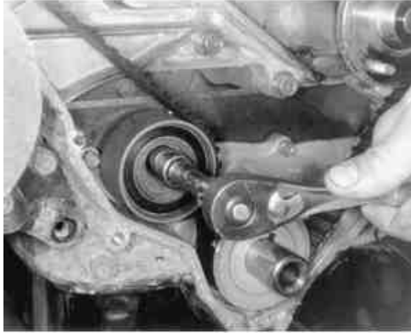
Fig. 16: Note the proper belt routing during removal
