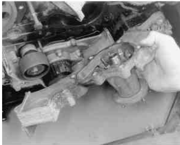
Fig. 19: Removing the timing belt tensioner assembly
