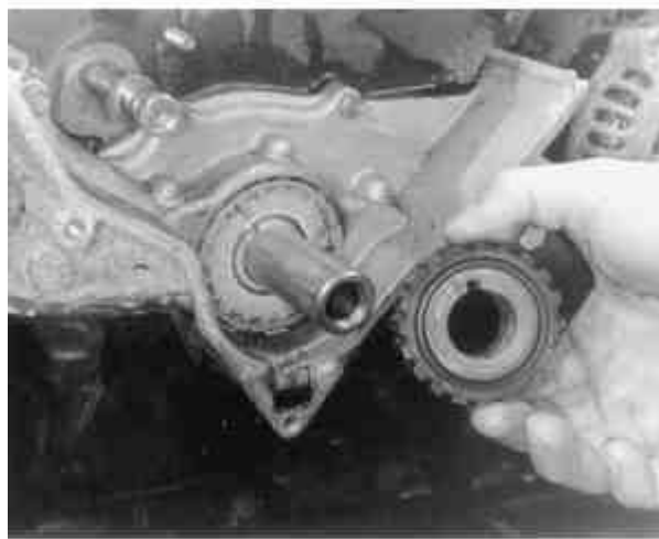
Fig. 6: Remove the oil pump cover to gain access to oil pump body — 6-cylinder engines
