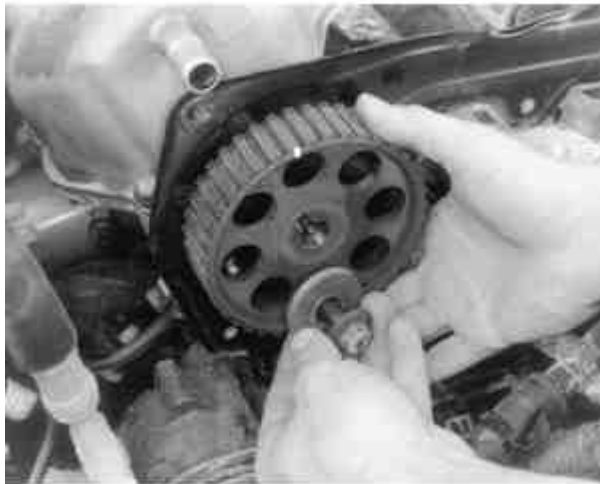
Fig. 4: View of the camshaft pulley — note the timing mark on top of the pulley
